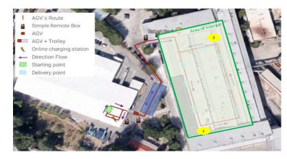
Real-time, cm-level AGV tracking with hybrid positioning
