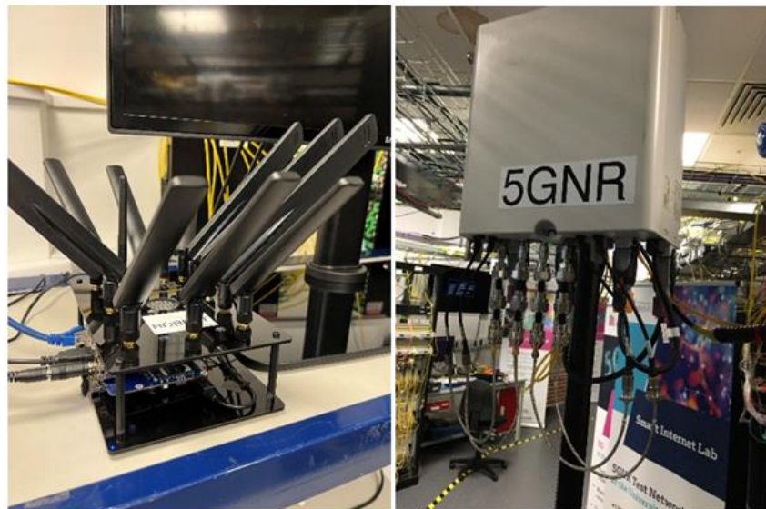
Figure 3-6 5G-CLARITY multi-WAT framework testbed setup at the Smart-Internet Lab -UoB
