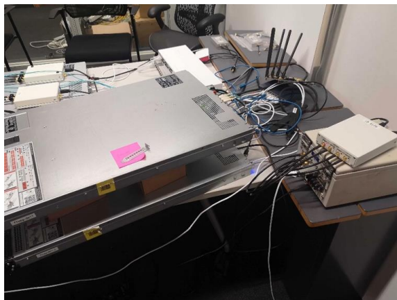
The testbed validation was done initially using the research RU National Instruments B210 Software Defined Radio (SDR), as shown in Figure 2-9. It was later validated with the commercial Benetel RUs that are also part of the multi-connectivity pilots.
