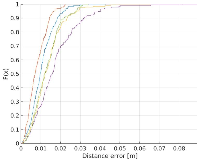
Figure 5-14. Empirical cumulative distribution function (eCDF) of the positioning error of the sub-6 GHz system
