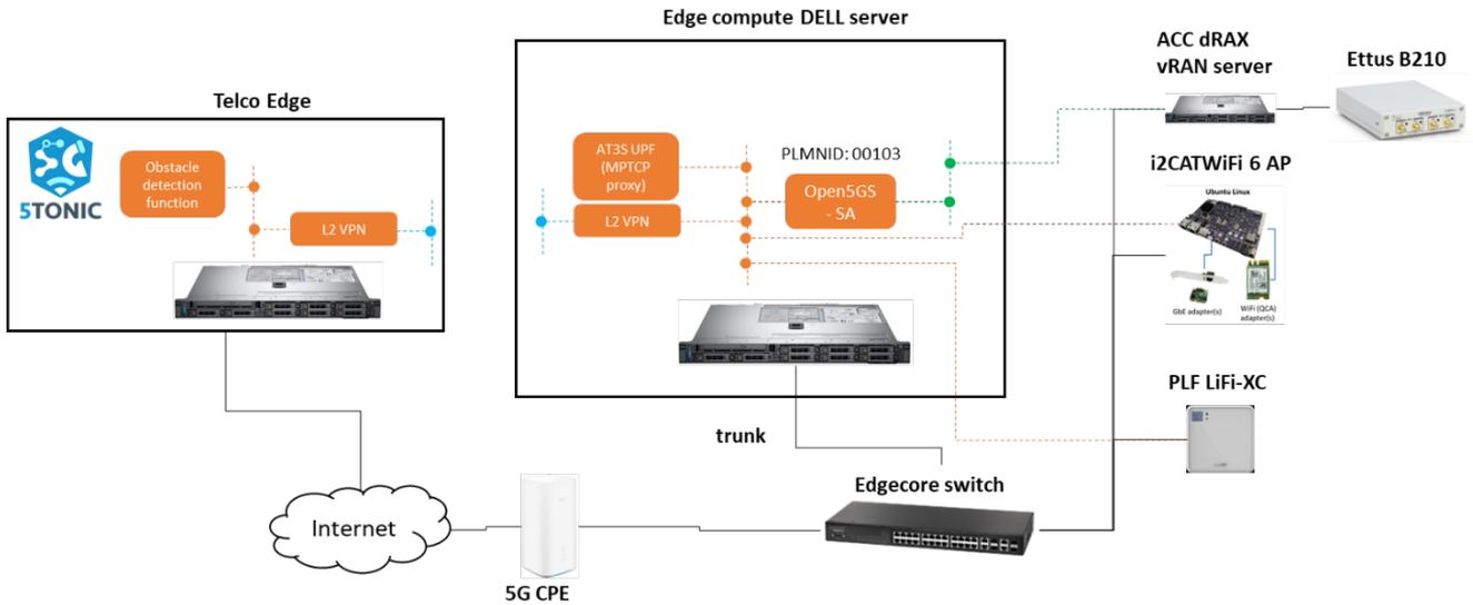
Figure 4-8. PNI-NPN slice design.
