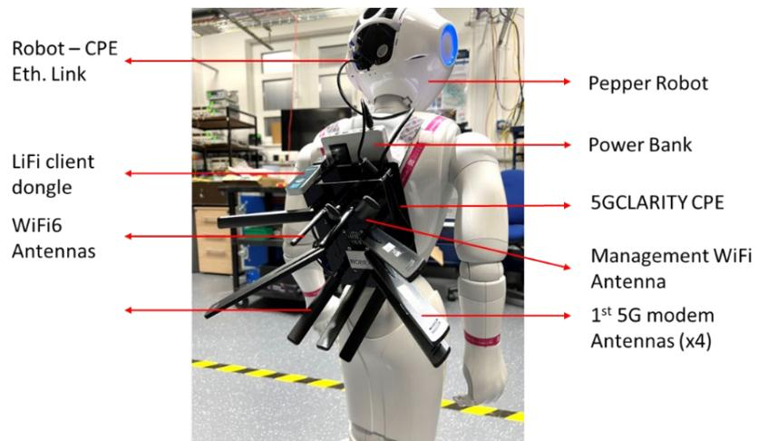
Figure 3-3. Guide Robot with 5G-CLARITY CPE.
