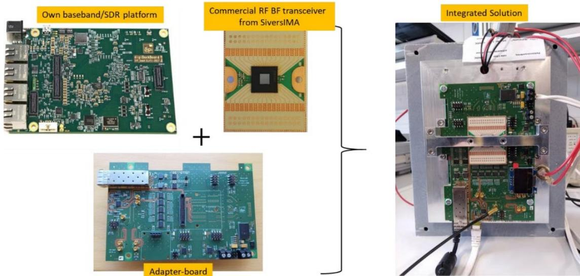
Figure 2-17. Sub-6 and mmWave localization integration.
