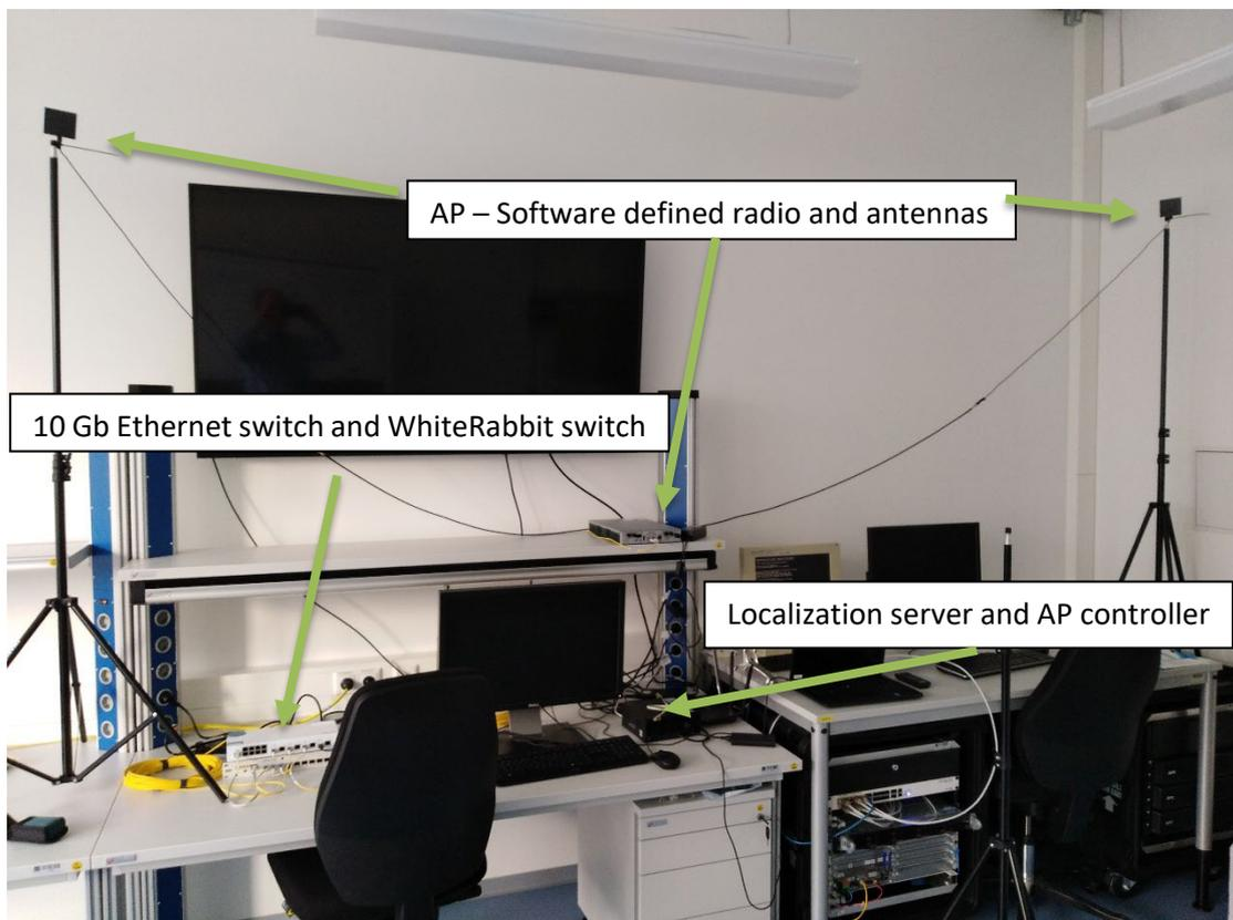
Figure 5-5. Sub-6 GHz localization setup - AN, localization server and AN controller.
