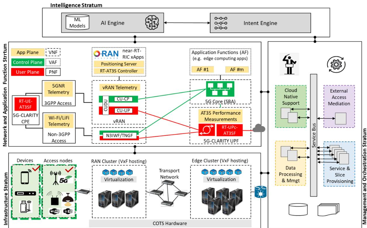
Figure 5-1. 5G-CLARITY system architecture to be used on UC2.2.
