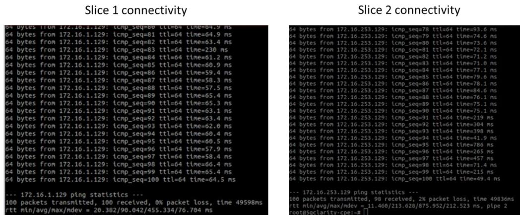
Figure 4-14. Connectivity from each UE to the core corresponding to their slice.
