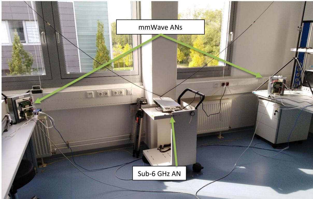
**Figure 5-6. mmWave ANs and a sub-6 GHz AN.**
