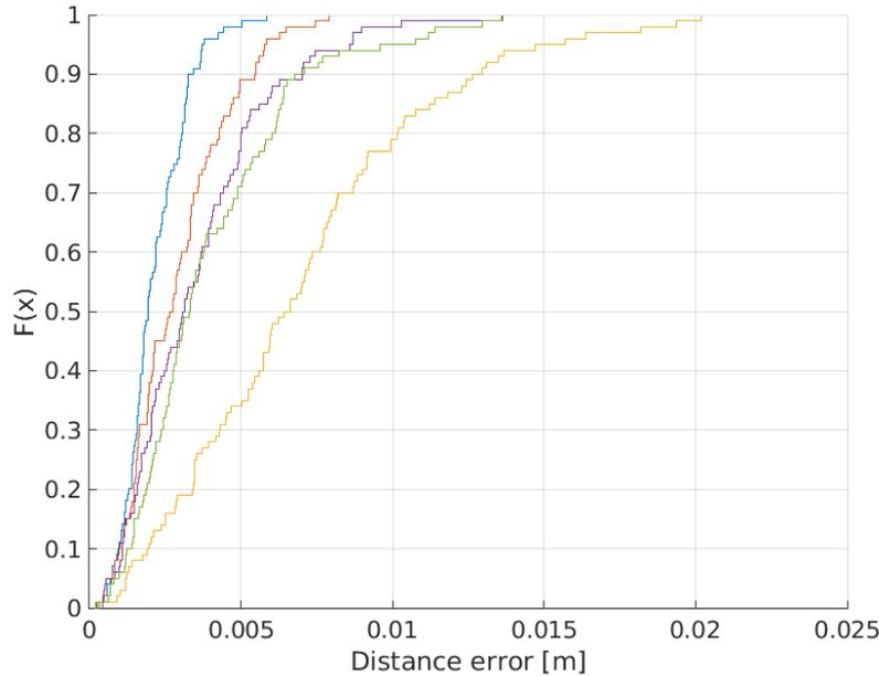
Figure 5-13. Empirical cumulative distribution function (eCDF) of the positioning error of the mmWave system
