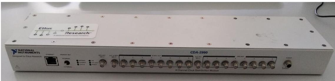
**Figure 2-15. OctoClock - initially used for synchronization of the anchor nodes**
