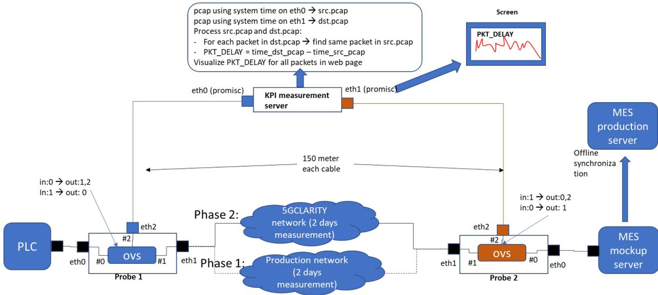
Figure 4-9. Design of one-way UL delay measurement toolkit.
