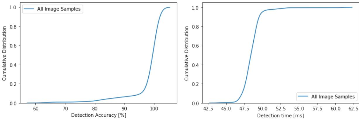
**Figure 4-19. Cumulative distribution of combined detection accuracy and detection time**
