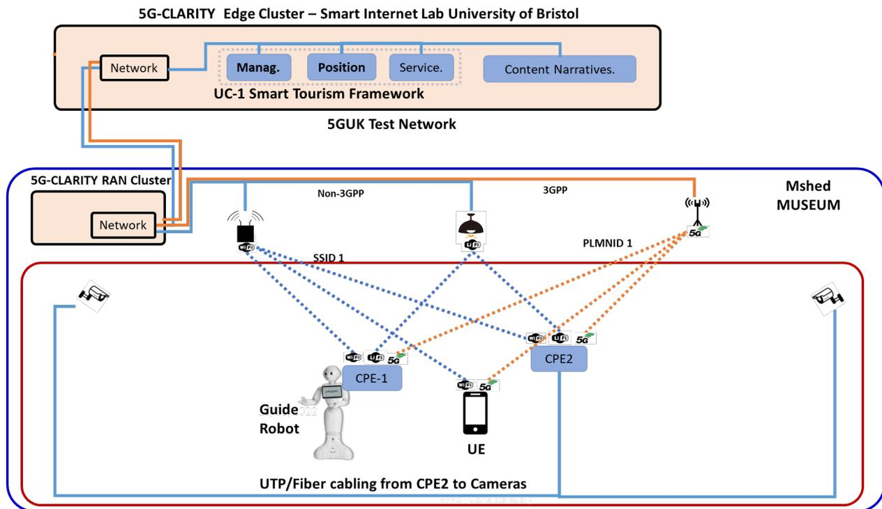
Figure 3-6. Proposed 5G-CLARITY UC1-Pilot Network Setup M-Shed.
