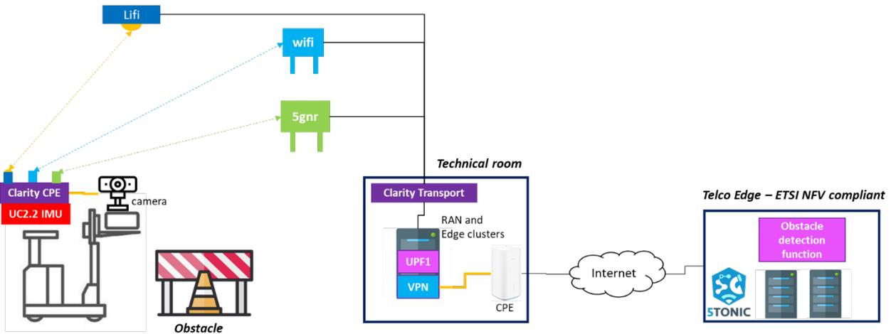
Figure 4-4 High-level design of PNI-NPN slice.
