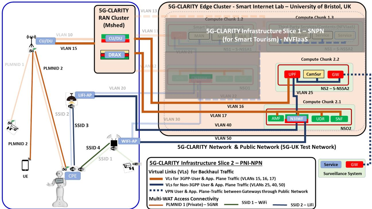
Figure 3-9. 5G-CLARITY PNI-NPN Infrastructure Slice 2 with Slaas for Narrative 2 demonstration.
