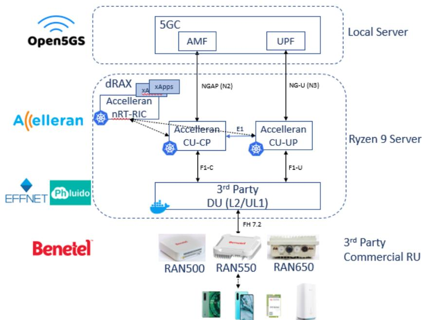
Figure 2-8. Final phase of integration with commercial Benetel RUs.
