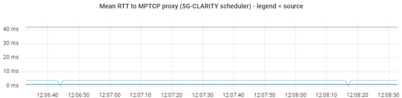
**Figure 2-27. Mean RTT between CPE and MPTCP Proxy for different RAT.**
