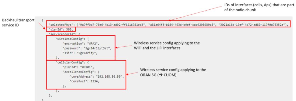
Figure 2-24. Example call to service provisioning endpoint of Multi-WAT non Real Time RIC.
