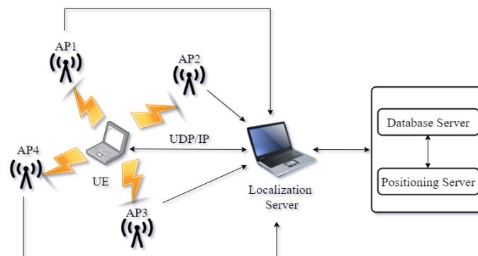
Figure 5-4. Laboratory testbed for testing the developed localization systems
