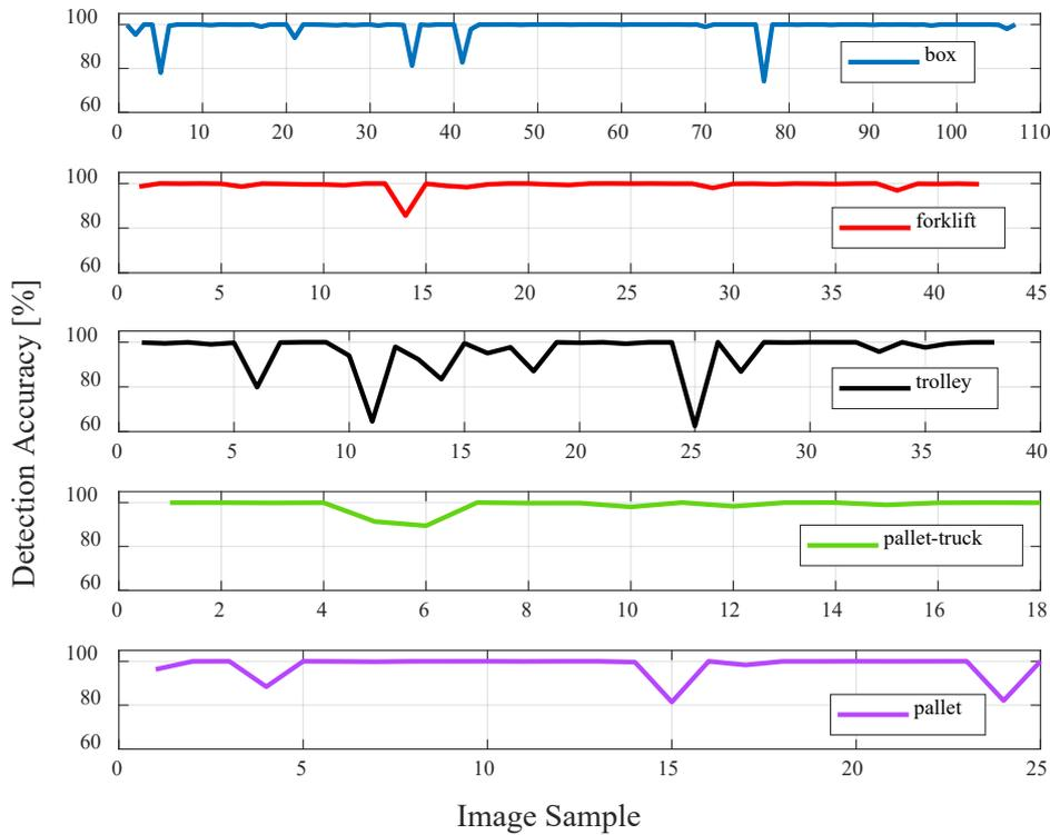
**Figure 4-18. Detection accuracy results according to object type**
