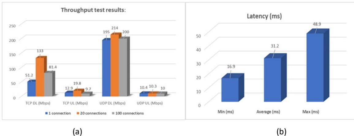
**Figure 3-12. 5G NR test results for (a) Throughput and (b) Latency performance of the ORAN 5G NR system.**
