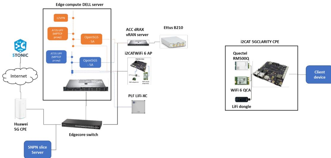
Figure 4-5. UC2.1 laboratory testbed at i2CAT.
