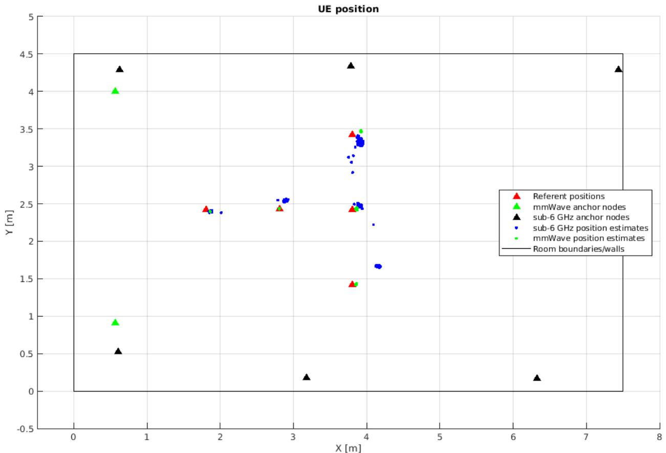
**Figure 5-11. Position estimates for the static scenario**
