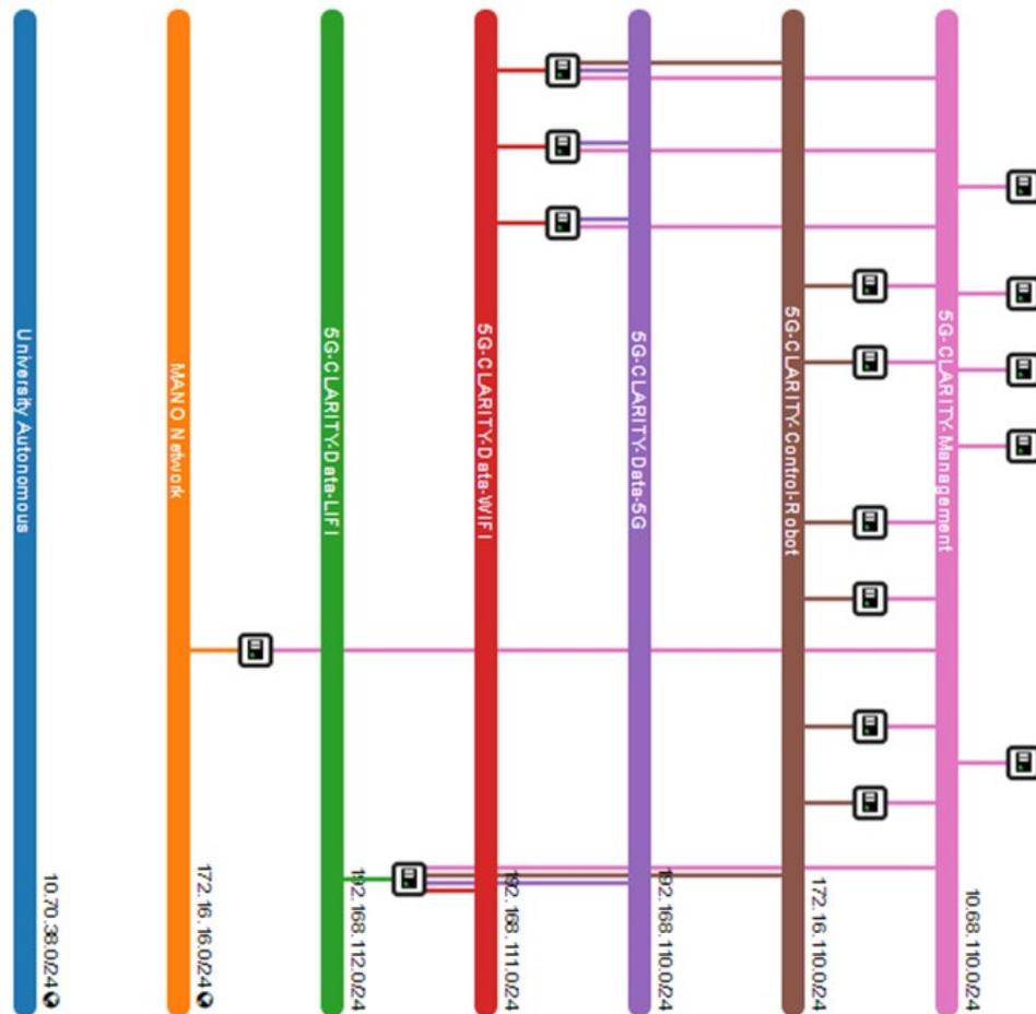
Figure 2-21 An illustration of the network topology describing the VM inter-connection and technology solution integrated for UC1 pilot site
