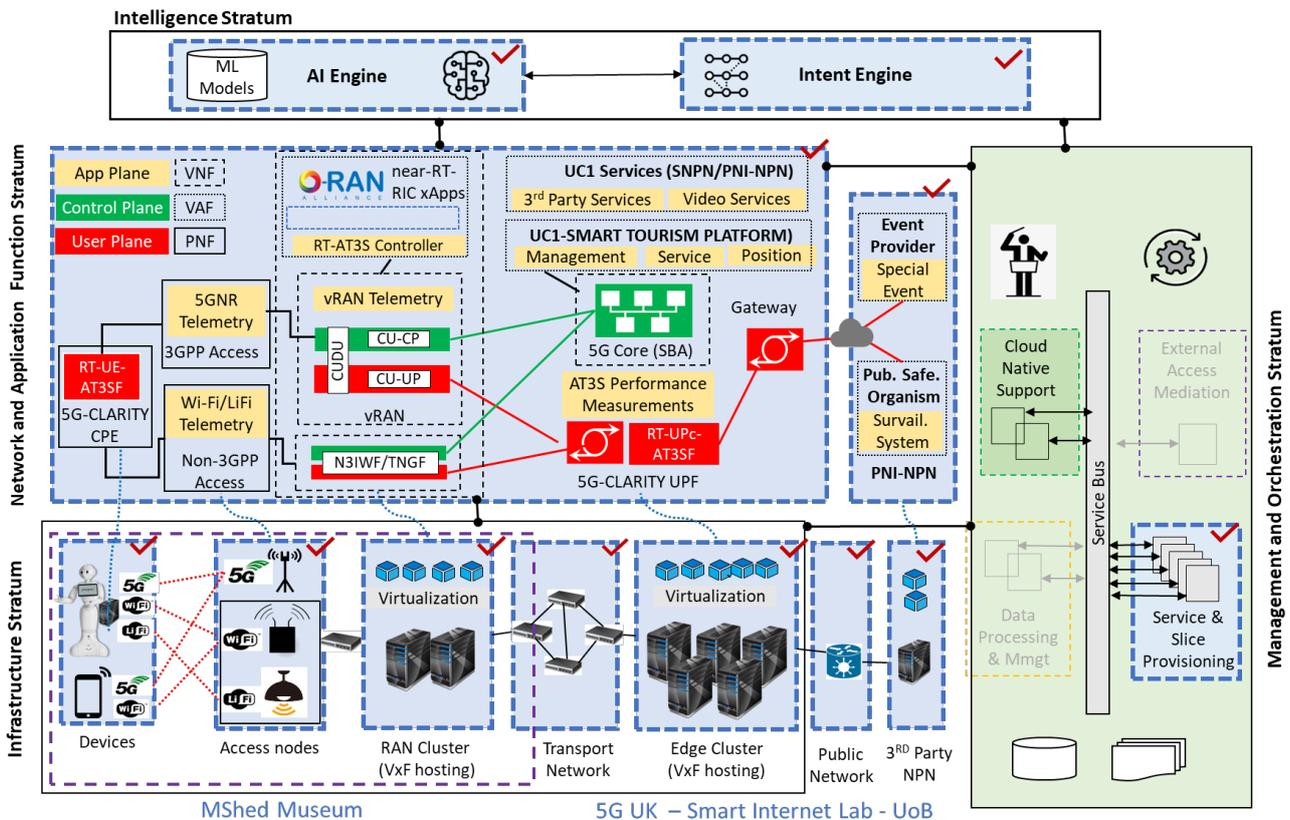
Figure 3-1. 5G-CLARITY system architecture to be used on UC1.
