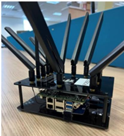
a) Main UC1 CPE based on Single Board Computer
