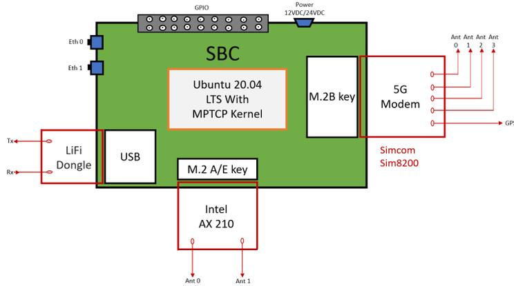
**Figure 2-2. Schematic view of the 5G-CLARITY UC1 CPE internal hardware design.**
