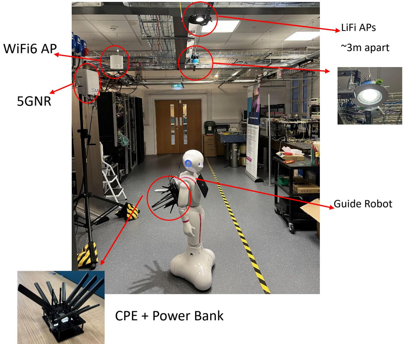
Figure 3-11. 5G-CLARITY UC-1 Lab Setup Smart Internet Lab.
