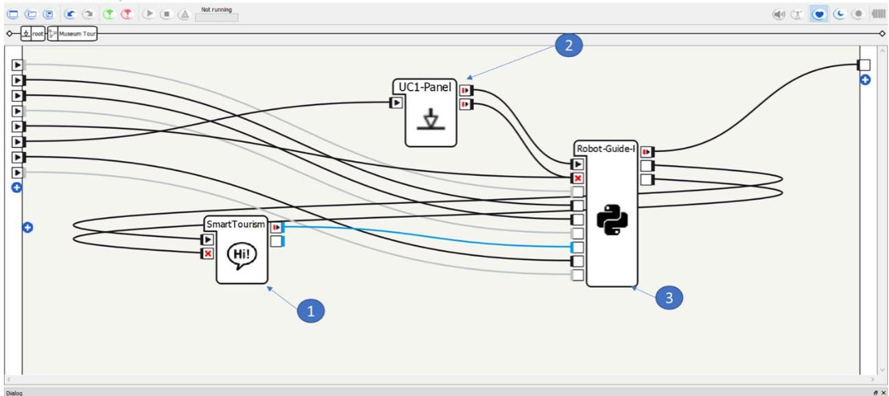
Figure 3-5. First Release of UC1-Smart Tourism Framework APIs written in Python 2.6 and C++ and deployed on IDE-Choregraphe 2.5.
