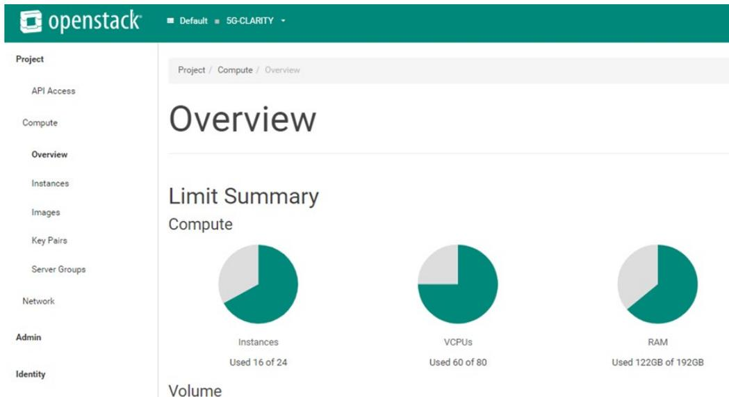
Figure 2-20. A sample summary of the allocated and used compute resources deployed in UC1
