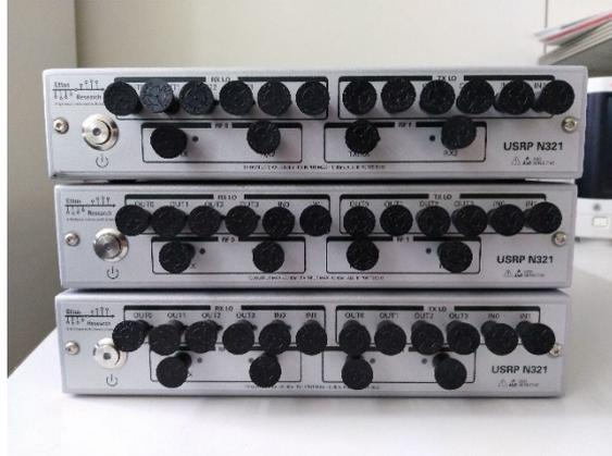
**Figure 2-14. SDR model USRP N321 for the Sub 6 GHz platform.**
