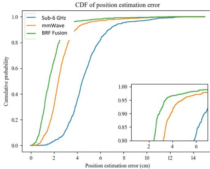
Figure 5-16. Performance of the overall simulated system, using the measured positioning technology parameters.
