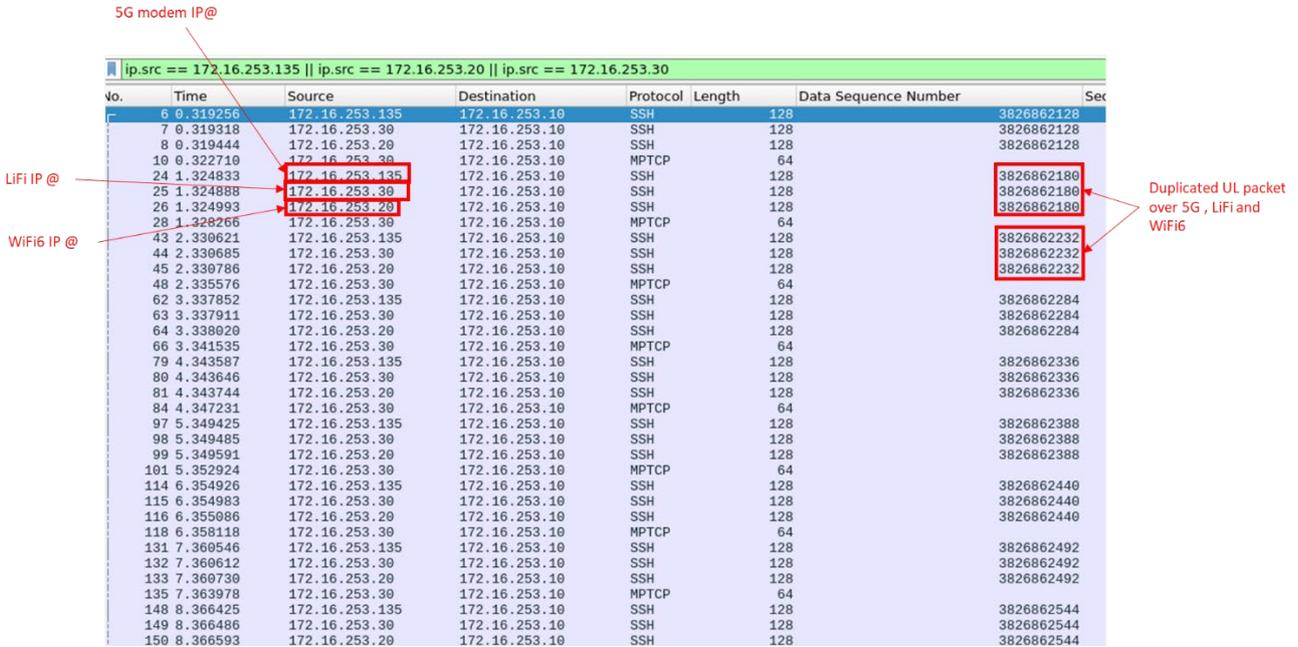
Figure 4-15. Capture of TCP packets generated by 5G-CLARITY CPE for UL measurement toolkit validation experiment
