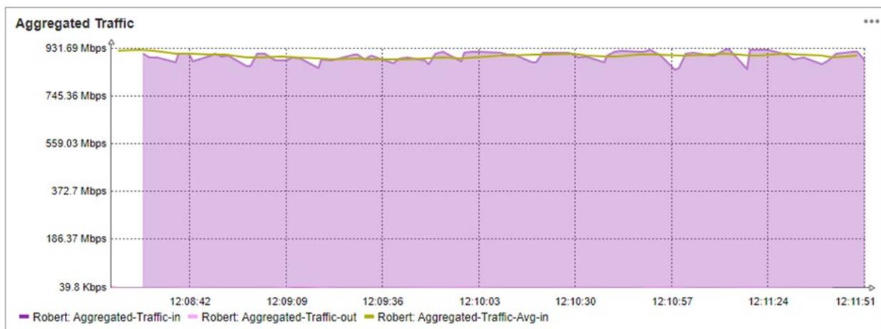
**Figure 3-14. Aggregated Download Throughput over 5G NR, WiFi-6 and LiFi with MPTCP running.**
