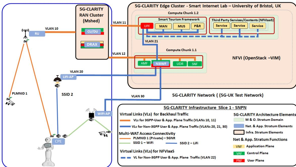
Figure 3-7. 5G-CLARITY SNPN Infrastructure Slice 1 with NFVlaaS for Narrative 1 demonstration.
