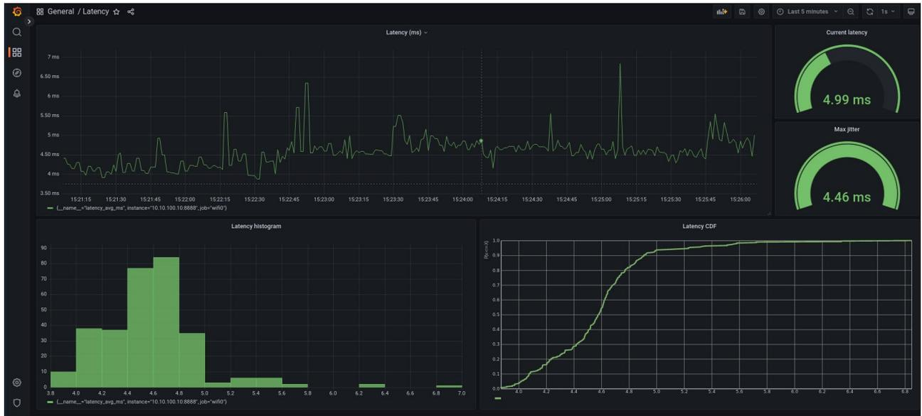
Figure 4-16. Measured UL network latency using our UL measurement toolkit
